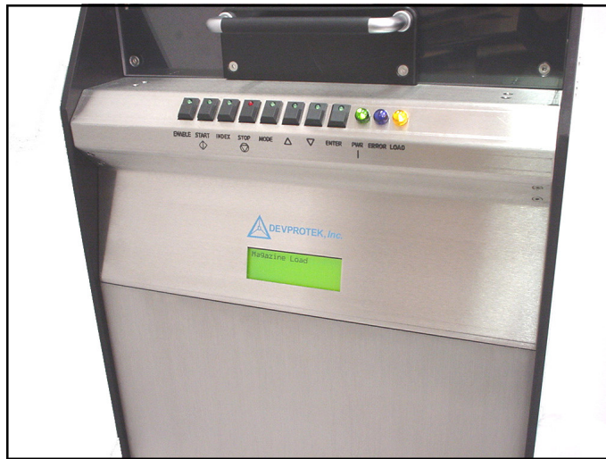
Push button controls with LCD user interface and status indicator lights.
